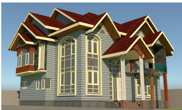
Multislope Designer Roof unfavourable for Solar Modules, insulation and maintenance
